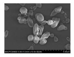
The Supercritical CO2 anti-solvent method (SAS) was used to obtain ultrafine CL-20 using Ethyl acetate as solvent and PEG-200 as surfactant. At 50  $^{\circ}$ C, 12 MPa and Mass percent concentration of 5%, ultrafine CL-20 was prepared. Result shows the surface of particles is smooth and the average particle size is 1.33 µm. There is little change in particle size distribution.
