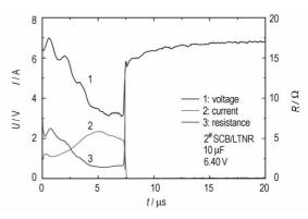
YANG Gui-li, ZHU Shun-guan, SHEN Rui-qi Chinese Journal of Energetic Materials, 2012, 20(4): 391 - 396 The electrical characteristics of SCB device were recorded when an ignition voltage was applied by a fast oscilloscope. The SCB firing mechanism was obtained by the analysis of resistance variation under different voltage inputs.
