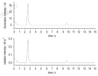
The Si/ Pb<sub>3</sub>O<sub>4</sub>/ BaSO<sub>4</sub> delay composition was prepared by coprecipitation method to improve the delay precision. The delay time and burning rate of the delay compositions were measured by photoelectric test system.
