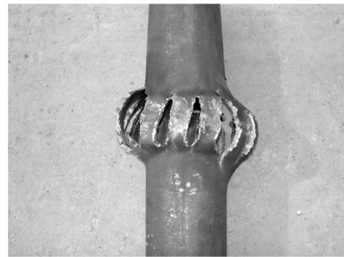
a. The shaped jet cutting the steel pipe (bottom)
