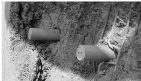
a. penetration of test projectiles into concrete target
