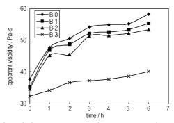
In the rheological characteristics test, the apparent viscidity and yield value of the raw boron powder (B-0) with HTPB increases rapidly with mixing time increasing, and gelates in 24 hours. B was neutralised respectively with ammonia in gas phase (B-1), in liquid phase (B-2) and with sodium hydroxide solution (B-3). The rheological characteristics of B-1, B-2 and B-3 with HTPB are improved. The apparent viscidity and yield value of B-3/HTPB mixture almost don't increase.
