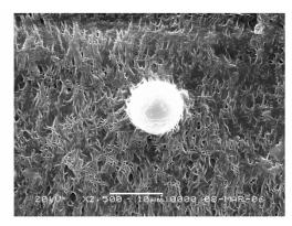
TANG Gen, GUO Xiang, PANG Ai-min, ZHENG Jian Chinese Journal of Energetic Materials, 2007, 15(4): 356-358 Spherulite of polymer generated after simple tension of PEG/N-100 matrix is observed by SEM. The matrix is of high Young's modulus, great yield stress and elongation percentage of fracture.
