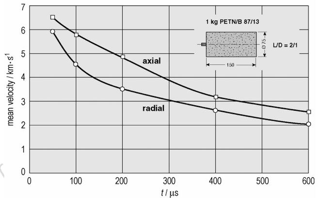
Fig. 10 Mean axial and mean radial velocities as a function of time delay
