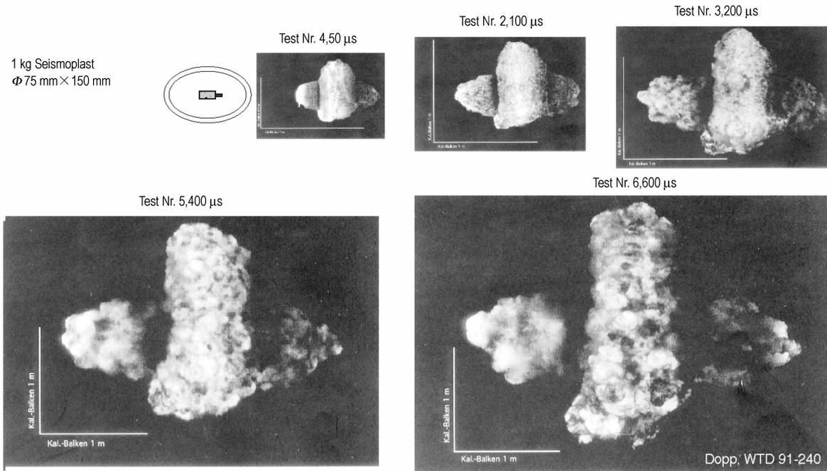
Fig. 7 The calibration bars have 1 m length. The five frames are now compared with the same magnification. The charge in the same scale to this frames are given in the upper line on the left in the circle
