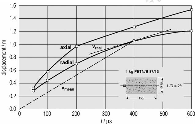
Fig. 9 Definitions of the mean velocities defined as a displacement divided by the delay time and the real velocity which is an tangent to the curves
