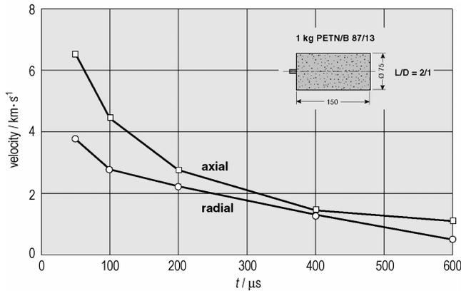
Fig. 11 Real axial and real radial velocities as a function of time delays
