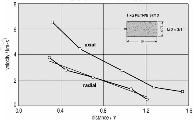
Fig. 12 Real axial and real radial velocities as a function of distance to the detonating cylindrical charge
