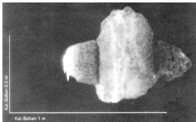
Fig. 2 Expansion of 1 kg detonating Seismoplast (PETN/binder-system 87/13) in cylindrical form of 150 mm length and 75 mm diameter, initiated in the axis from the right sight.
