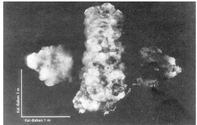
Fig. 6 Expansion of the reaction products of the same charge after 600  $\mu\text{s}$  delay time, but with 0.2  $\mu\text{s}$  exposure time
