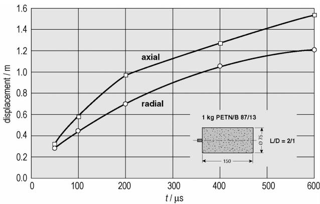
Fig. 8 Axial and radial expansion distance as a function of the delay times
