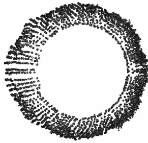
图 6 90°偏三线起爆的破片场 Fig. 6 Fragment field initiated in three generatrices (90°)
