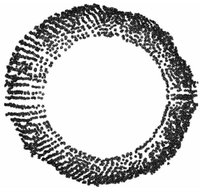
图 5 90°偏两线起爆的破片场 Fig. 5 Fragment field initiated in two generatrices (90°)
