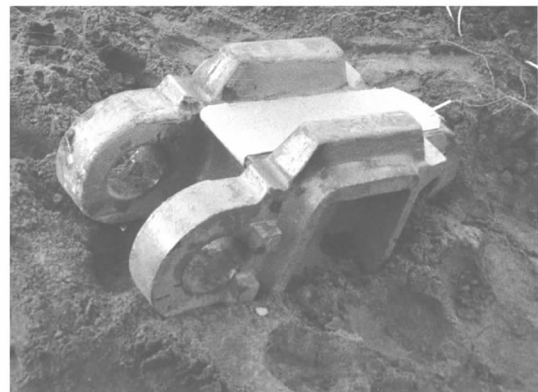
Fig. 3 Track link with a layer of plastic explosive stuck to the surface of rolling track wheel
