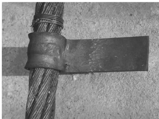
Fig. 6 General view of the ring clamped on steel cable by explosion method
