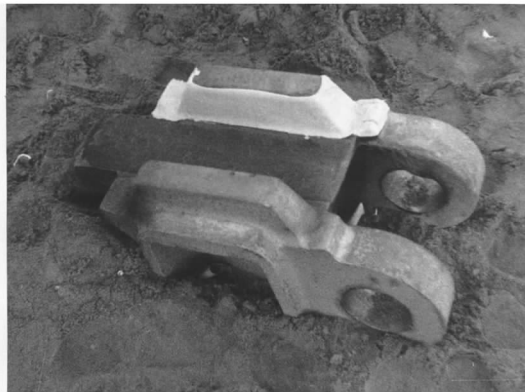
Fig. 4 Track link with layers of plastic explosive stuck to the lateral surface of the shelf
