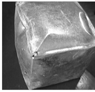
图 6 毁伤增强型破片对铁制箱体的内爆打击效果 Fig. 6 Exploding effect inside iron cases by a damage enhanced fragment
