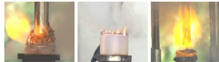
b. the combustion image of porous electrode, porous mesh electrode and screen electrode
