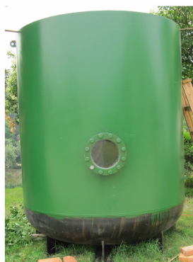
Fig. 1 The container for the underwater explosion experimental
