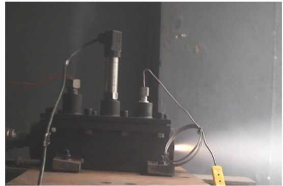
b. paraffin-based fuel ignite experimental device
