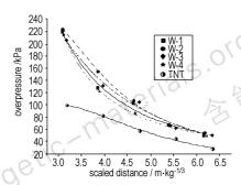
Composite explosives with good damage performance were studied. Explosives were composed of NH<sub>4</sub>NO<sub>3</sub>, Al powder, liquid function additive and sensitizer.
