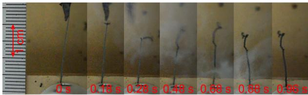
a. self-sustaining combustion of 2# fiber propellant
