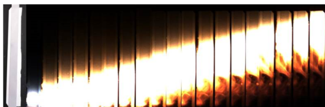
图5 用高速摄影测得 Al/CuO x 复合薄膜的燃烧速率 Fig.5 The burning rate of Al/CuO x multilayer films obtained with high speed camera
