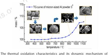
micron-Al powders in air were investigated by TG/DTA. Three kinds of particle sizes of aluminum powder were heated up to 1110  $^{\circ}$ C at 10 K  $\cdot$  min<sup>-1</sup> heating rate in air. SEM and XRD were used to determine the evolution of the Al samples by observing the products collected at selected temperatures. The kinetic parameters of the oxidation reaction were calculated by Satava-Sestak integral method.
