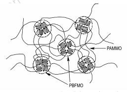
The fluorine-containing PAMMO based thermoplastic elastomers were developed using PAMMO as the soft segments and the PBFMO preparing from a cationic polymerization as the hard segemnts to enhance its comprehensive properties. The molecular structure, relative molecular mass and mechanical properties of thermoplastic elastomers were confirmed by FT-IR, NMR, GPC, DSC, TG/DTG and universal testing machine, respectively.
