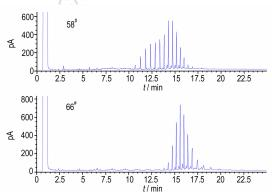
Chemical components of paraffin fuel for hybrid rocket were studied by gas chromatographic analysis. According to the law of carbon number and integrating the peak area, the carbon number distribution and percentage contents of the n-alkanes of paraffin fuels can be analyzed. Therefore, the relationship between the chemical components and combustion characteristics of paraffin fuels can be investigated.
